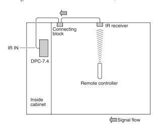
Connect the IR receiver to the DPC-7.4 as shown below.
